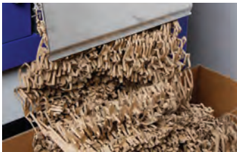
High bulk void fill from waste cartons
